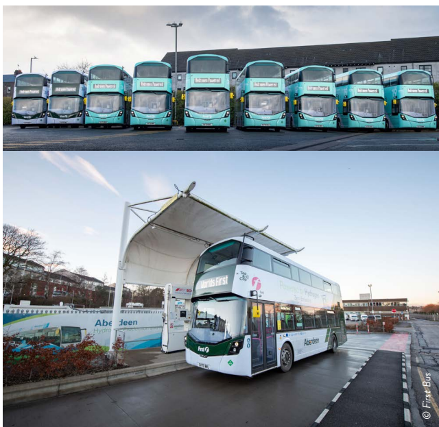
▶ Figure 4: Buses and HRS in Aberdeen, United Kingdom. Top: Part of the double-deck FCB fleet. Bottom: Bus refuelling.
